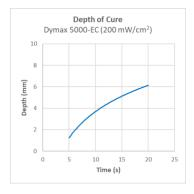
Full cure is best determined empirically by curing at different times and intensities and measuring the corresponding change in cured properties such as tackiness, adhesion, hardness, etc. Full cure is defined as the point at which more energy exposure no longer improves cured properties. Higher intensities or longer cures (up to 5x) generally will not degrade Hanarey light-curable adhesives.
