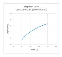
Full cure is best determined empirically by curing at different times and intensities and measuring the corresponding change in cured properties such as tackiness, adhesion, hardness, etc. Full cure is defined as the point at which more energy exposure no longer improves cured properties. Higher intensities or longer cures (up to 5x) generally will not degrade Hanarey light-curable adhesives.
