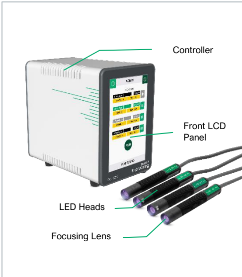
Figure 1. Main Components of the SC-225
