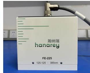
Figure 12. Plug Interconnect Cable into Emitter
