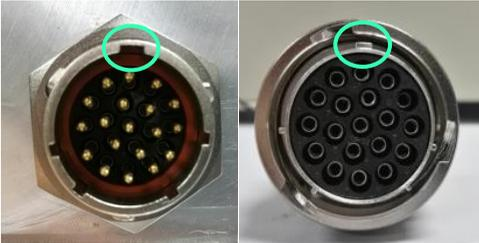
**Plugging the footswitch or light shield into the controller:**
