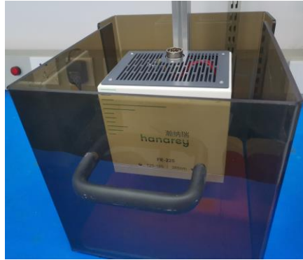
Figure 40. Mounting Stand (PN 88844, Emitter not Included)
