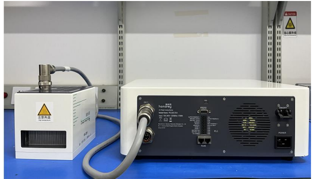
Figure 6. Interconnect Cable Installed
