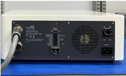
Figure 11. Plug Interconnect Cable into Controller
